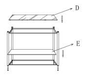
4. Carefully place the Tempered Glass onto the Top shelf, and then put the Marble onto the Bottom Shelf.
